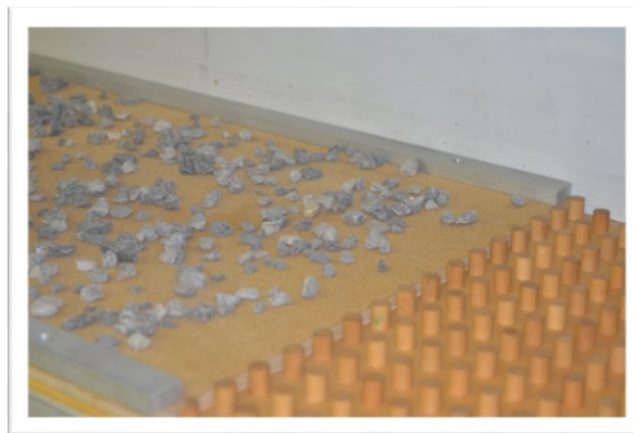
Figure 2-5 Transition from wooden dowelling to sparse stone.
