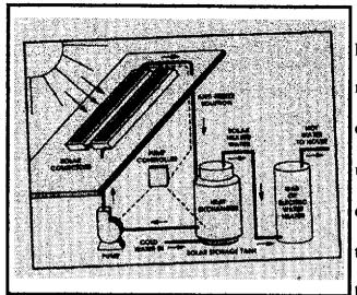
Active solar heating differs from passive solar heating in that it involves the mechanical transportation of collected solar energy to a storage or distribution system for use. Active solar heating employs flat-plate collectors located on a south-facing rooftop that capture the sun's energy in a heat-transporting fluid, usually water, that is
