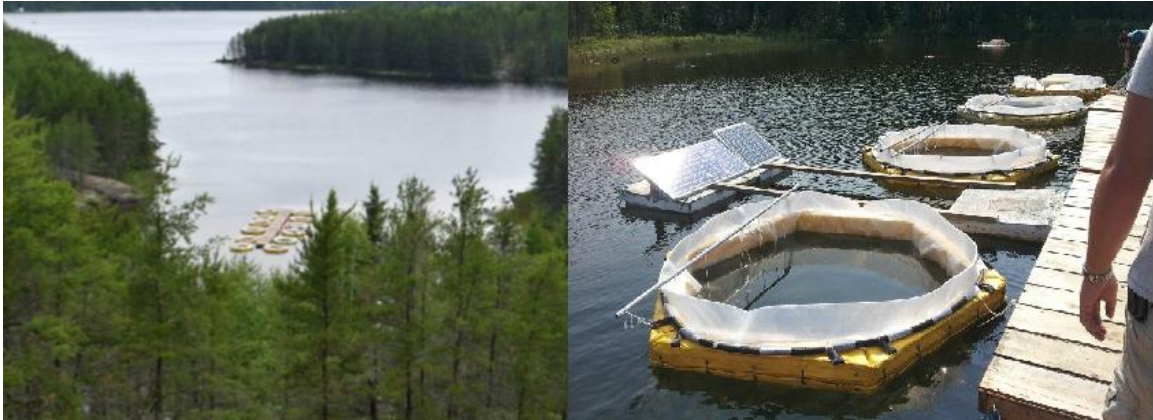
Figure 1: Aerial view of the mesocosm study set up in L239 (left). Mesocosms attached to docks (right).
