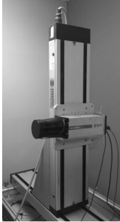
Figure A.2: The Dantec TM 2D Laser Doppler Anemometer
