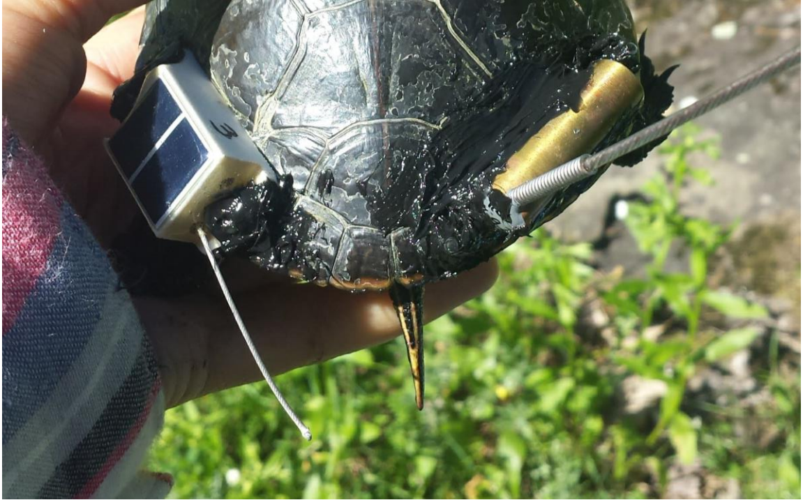
Figure 1: Accelerometer (left) and VHF transmitter (right) bolted onto the rear carapace margin of a Painted turtle.
