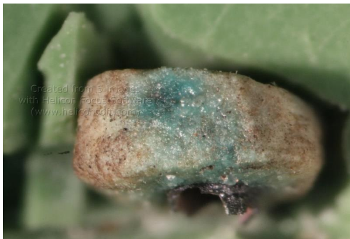
Figure 4.11: Bead 73. Application glazed bead with glaze applied through both immersion and painting, subsequently being fired at 1000 c for one hour. Example of uneven glaze absorption.
