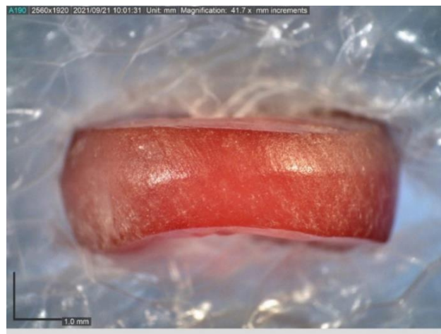
Figure 6.2 5076.003 with visible linear traces from grinding.
