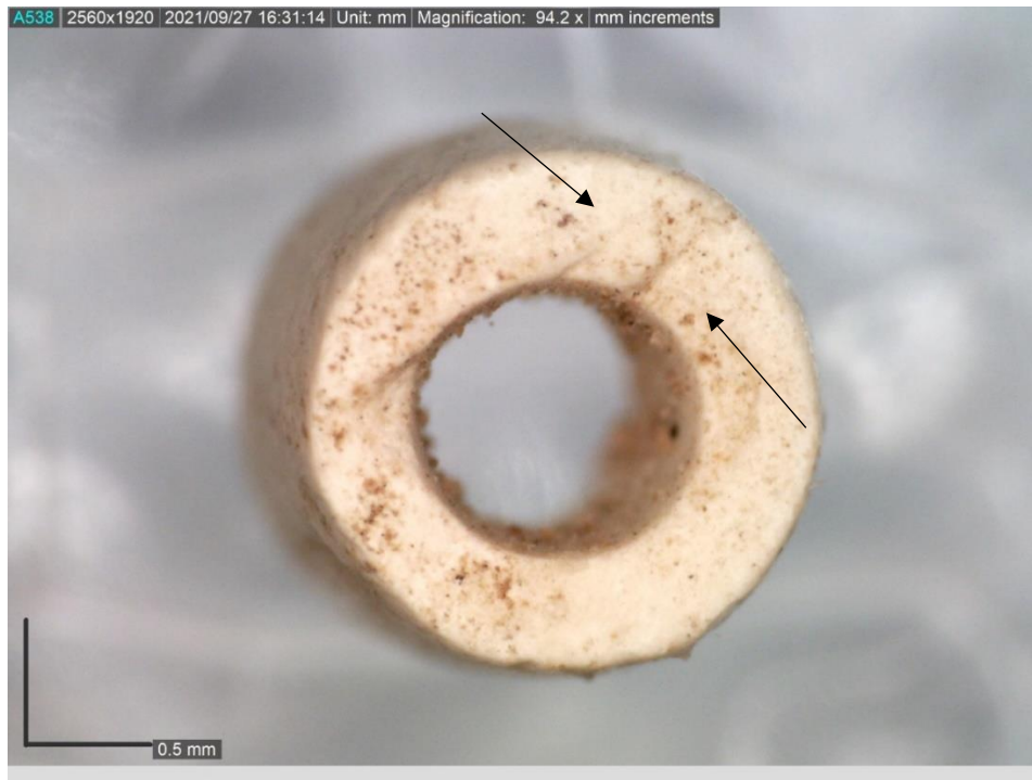
Figure 5.30 5108.001-020 with a concavity appearing on only one side of the drill hole.
