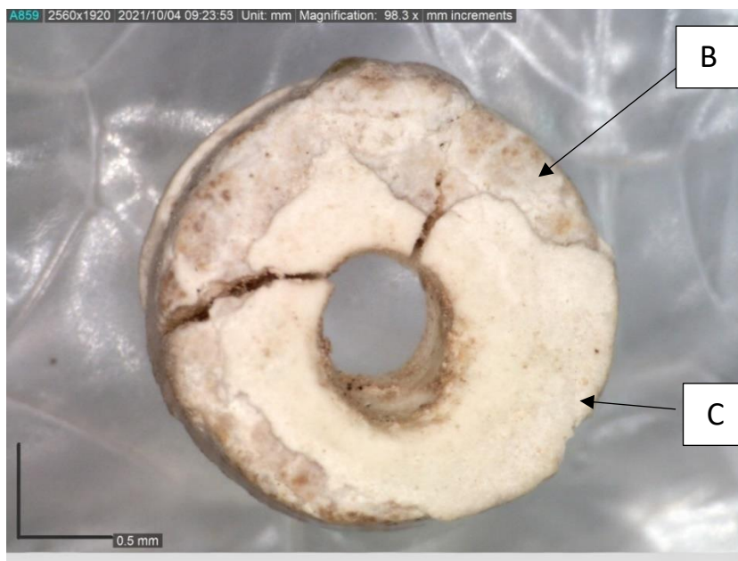
Figure 5.19 5070.004-074 with solid outer glaze layer (C) appearing superimposed above the white film transition layer (B)
