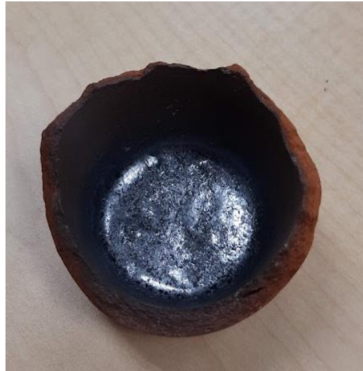
Figure 4.16 Unsuccessful cementation glazing attempt where beads were fired at 1000 c for one and a half hours. The glazing powder in this experiment transformed into a solid glassy mass.
