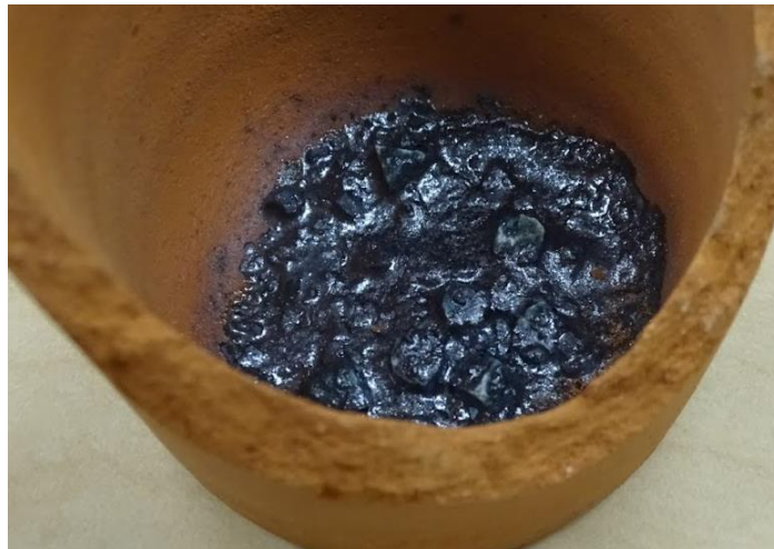
Figure 4.15 Unsuccessful cementation glazing where beads were fired at 1000 c for an hour. This resulted in the powder hardening making it impossible to extricate the beads.
