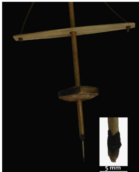
Figure 2. 16 Reconstruction of a bow drill with a hafted flint splinter (Reproduced from Groman-Yaroslavski and Bar-Yosef Mayer 2015: 86).
