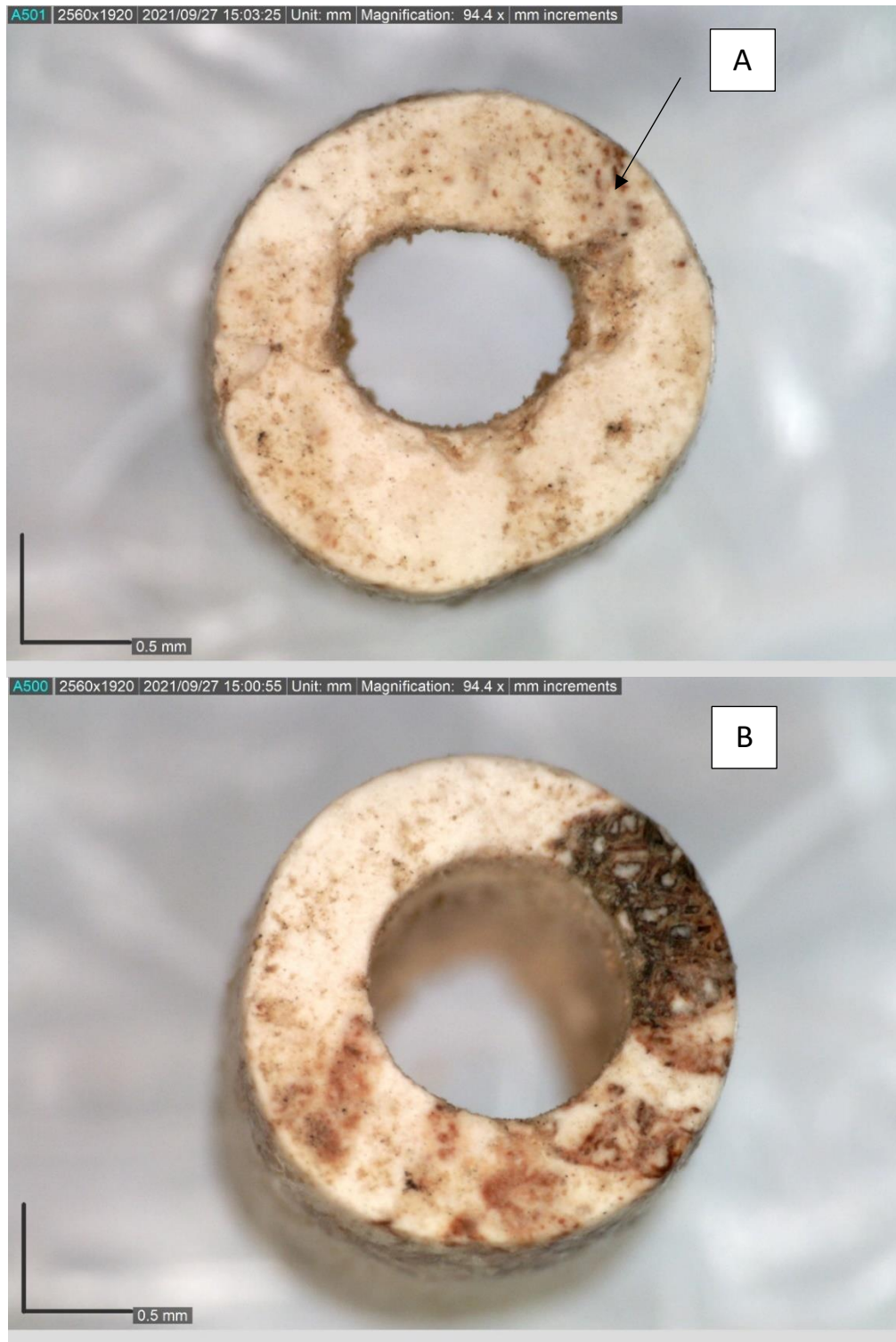
Figure 5.31 5108.001-026 (A) elliptical drill hole opening exhibiting chipping (B) circular drill hole opening without chipping.
