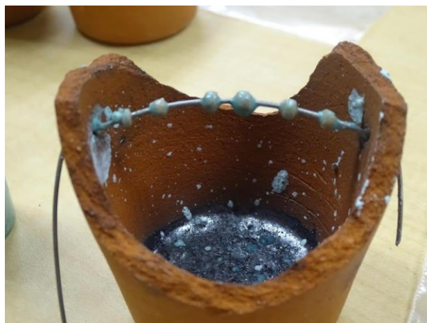
Figure 3. 8 Beads coated with application glaze mixture and suspended with kiln wire.
