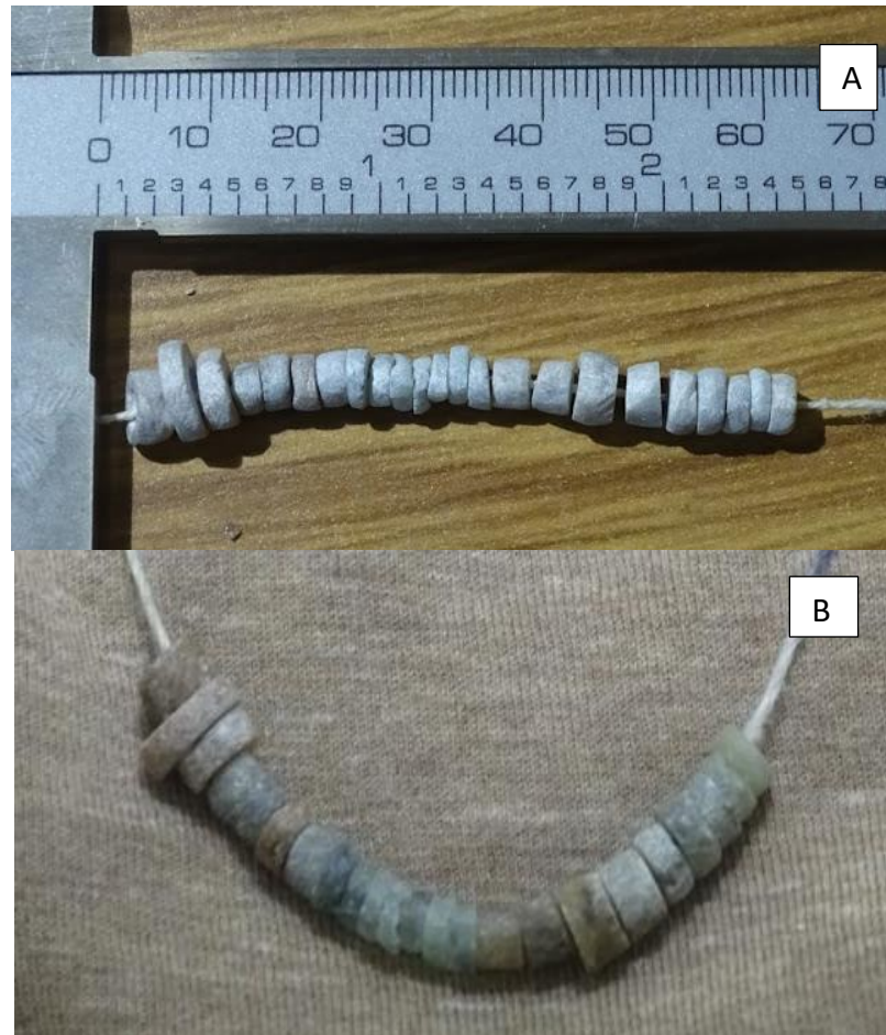
Figure 4.8 a. Experimental talc beads before being worn. B. Experimental talc beads after being worn for one week.
