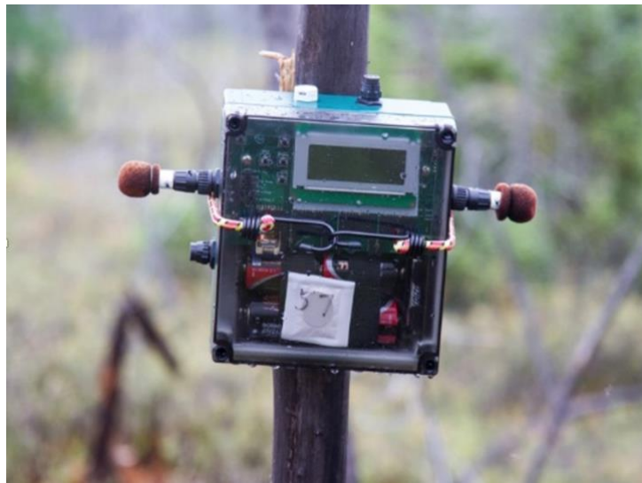
Figure 2.1. Example of a Wildlife Acoustics, Inc. ARU showing microphones on opposite sides of device.
