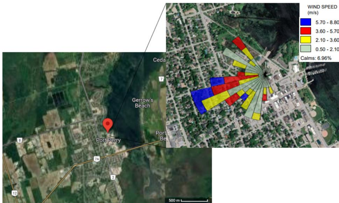
Figure 3.1 - Location of the ambient air sampler in Port Perry, next to Lake Scugog. The wind rose shows the wind direction and speed during November 1–5, 2021 mainly coming from the south-west.
