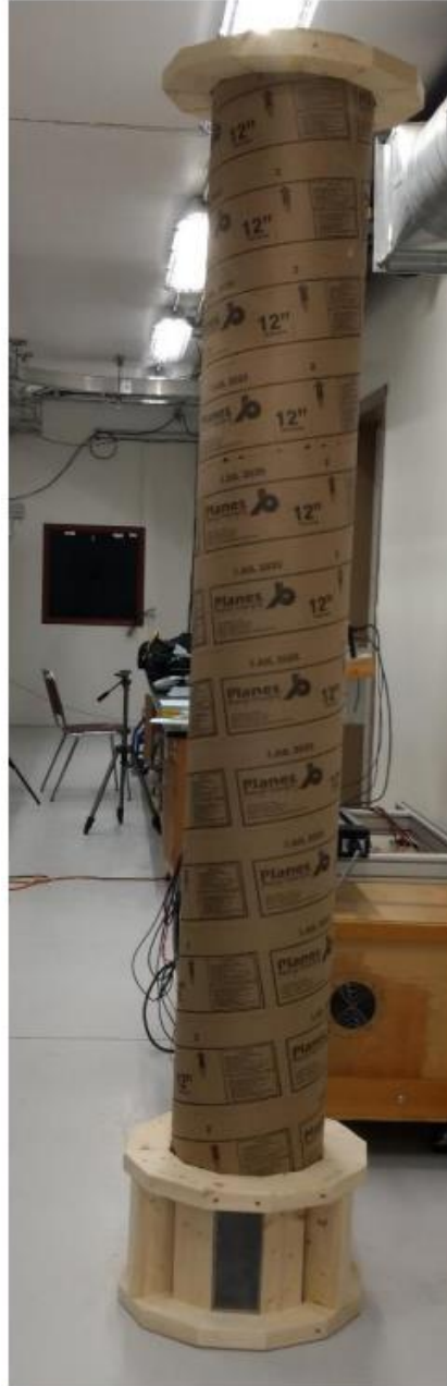
Figure A3.2- Photograph of the fall column constructed to determine the settling velocity of polyester microfibers, showing the base and top cover of the fall column (see Figure 3.2).
