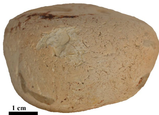
Figure 4.10: The surface of S3F3 after 60 minutes of bone abrasion.
