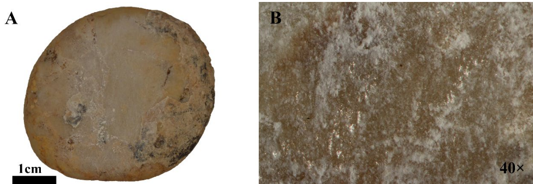
Figure 4.30: Residues on the surface of S7F1 after 60 minutes of shell abrasion. A) Reflective shell residues at the naked-eye level. B) Reflective film with a linear orientation.
