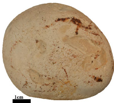
Figure 4.28: The surface of (S3F2) after 240 minutes of hide softening.
