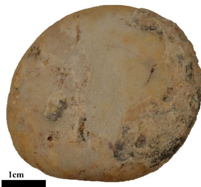
Figure 4.31: The surface of S7F1 after 120 minutes of shell abrasion.
