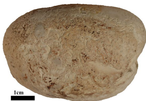
Figure 4.34: The surface of S3F5 after 120 minutes of wood abrasion.
