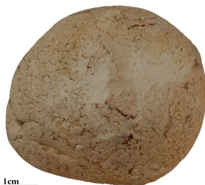
Figure 4.13: Alteration of the surface of S3F1 after 60 minutes of bone abrasion.
