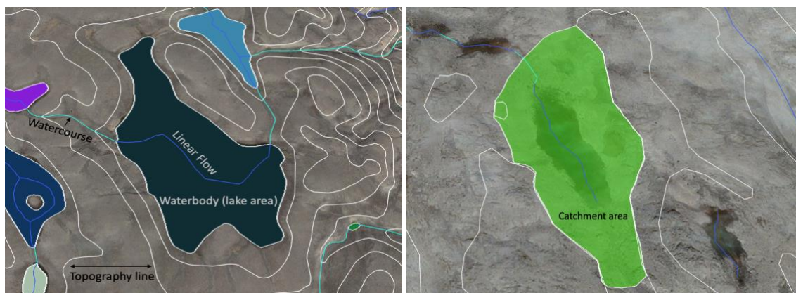
Figure C1: Google Earth Pro images of the layers (waterbody, water course, linear flow and topography; left), and catchment area (right).
