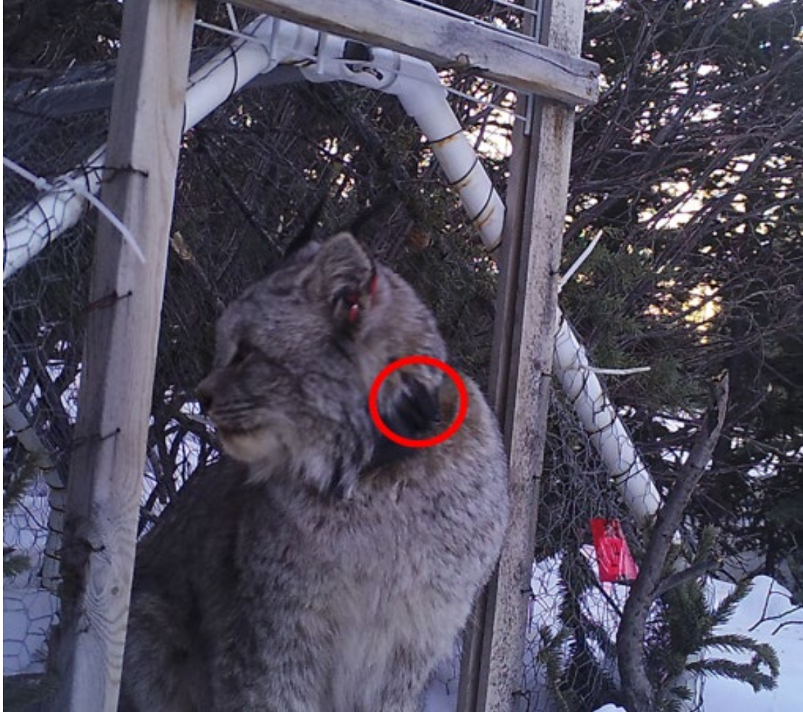
Figure A-A2: Location of audio recorder attachment when deployed on Canada lynx. The recorder sits just above the battery for the GPS unit (red circle). In this photo, the collared lynx is exiting a lynx trap.
