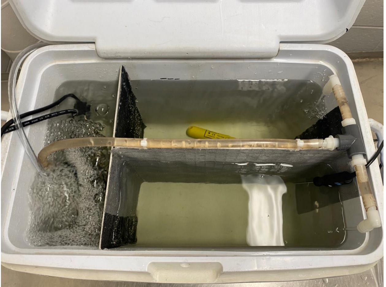
Figure A2. Partitioned cooler modified for fry CT_{max} arena. Pumps and heaters were separated from the fish by a mesh screen allowing flow through. An additional pump filtered warm water evenly throughout the sections. An airstone was used to maintain 100% oxygen saturation (monitored using a YSI; YSI ProSolo ODO Optical Dissolved Oxygen Meter https://www.yisi.com/prosolo-odo ), and temperature was recorded using an RBR ProSolo Temperature logger ( https://rbr-global.com/ ).
