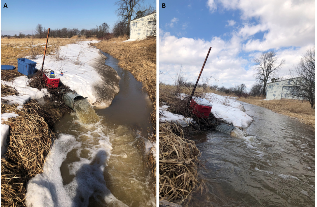
Figure 6-6. Visual representation of the change in Mystery TD discharge due to melting snow on March 6, 2022, where A) was taken at 11:00 am and B) was taken at 1:30 pm.
