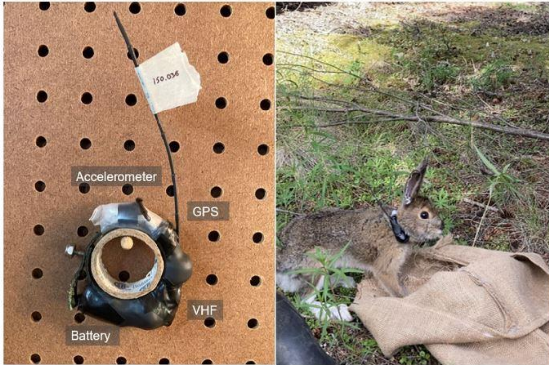
Figure 1 Radio-transmitter collar combining GPS, accelerometer, and VHF unit for monitoring movements and classifying behaviours of snowshoe hares. Photo credit: H. Miller.
