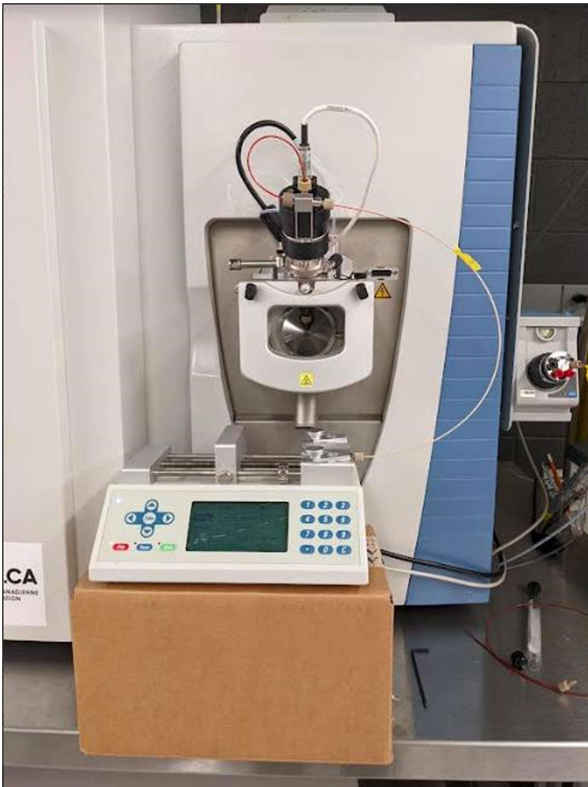
Figure 2.1: Syringe pump set up for HRMS analysis.
