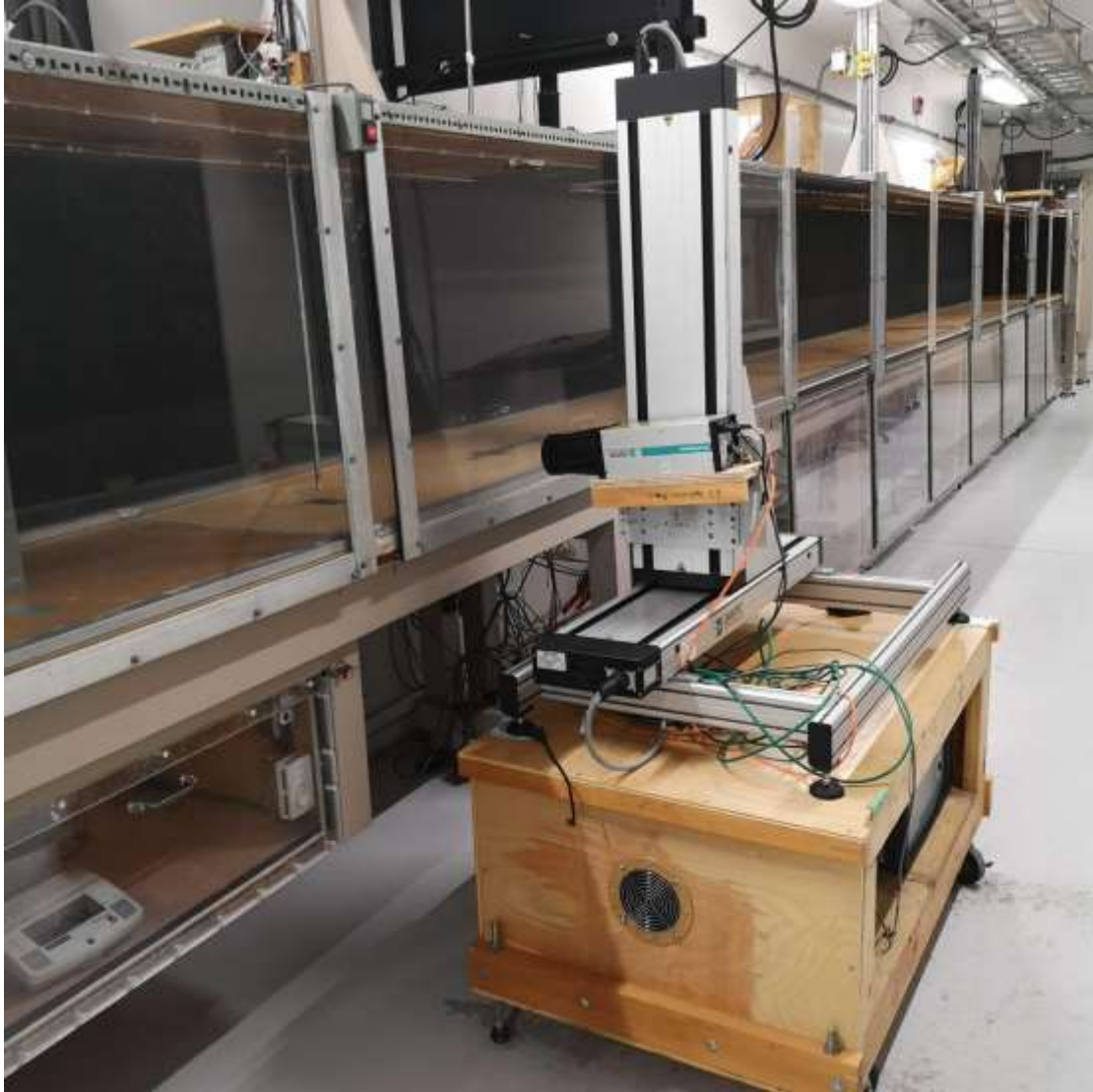
Figure 2.6: LDA Flow Explorer laser head, traverse mounted and on top of mobile compartment within which is stored the processor. The LDA is positioned normal to the airflow within the tunnel, where the intersection of the lasers (sampling volume) is situated approximately in the middle of the tunnel.
