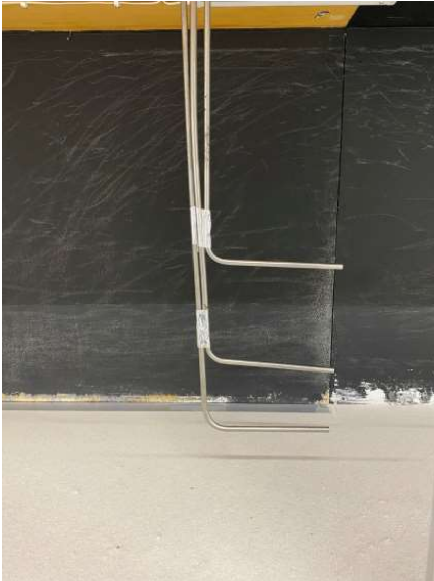
Figure 2.7: DustTrak intake tubes with an inner diameter of 3 mm, flow-aligned to allow for particulates to enter, at their fixed height (0.1, 0.2, and 0.3 m) above the sand bed. The tubes were taped together to ensure their positioning remained constant throughout the experiment.
