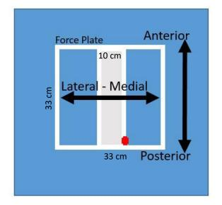
Overhead rendering of matted platform with embedded force plate.
