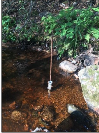
Figure 2.4 Adapted Hobo U20L logger design from Fogg et al. (2020) installed at H1.
