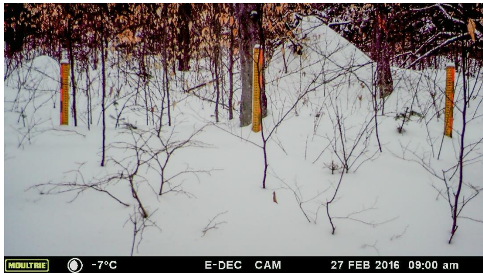
Figure 4.2: Example of trail camera and rulers for measuring snow depth at the deciduous site in the east region.
