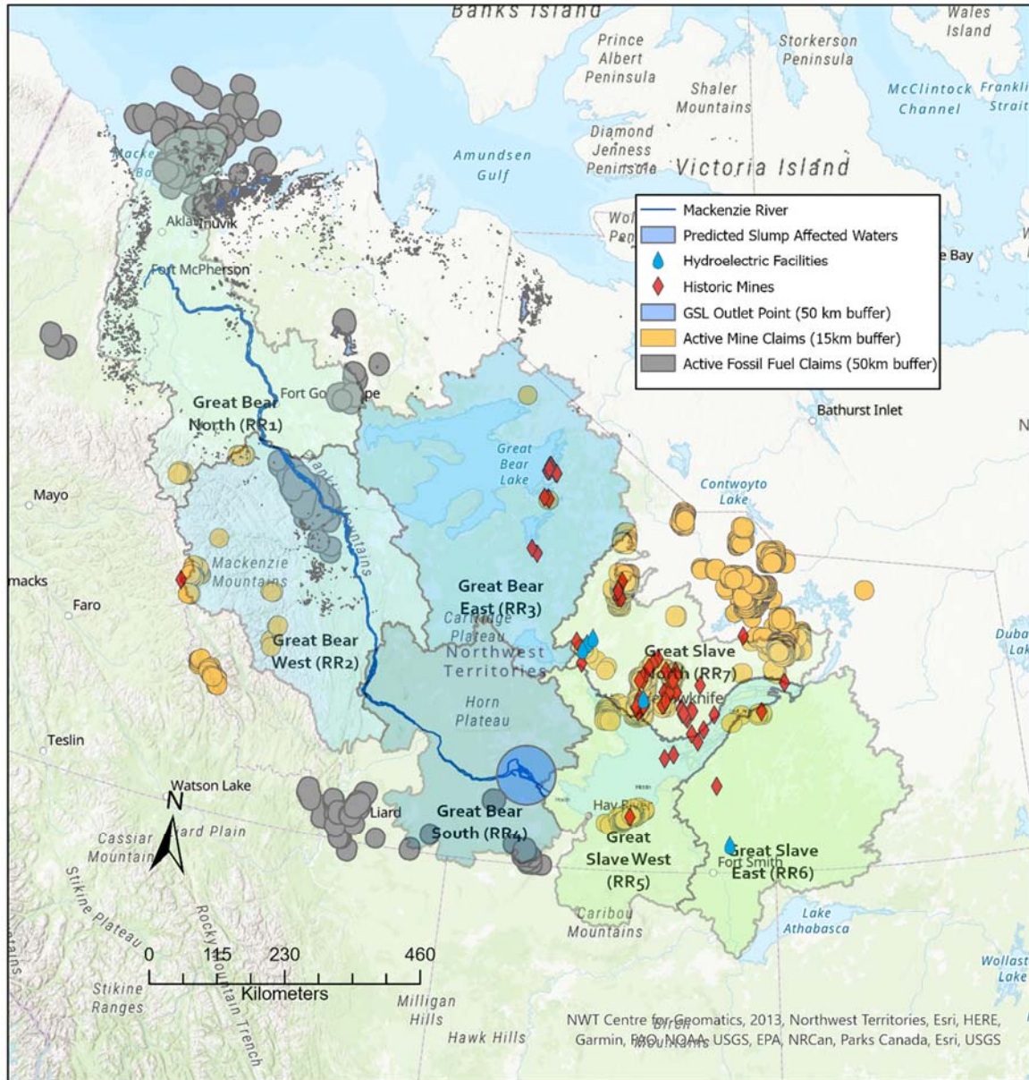
Supplemental Figure 13. The location of point sources considered in the GSL and GBS model frameworks. The polygon layers for the mining (orange circle) and fossil fuel developments (grey circles) represent a buffer layer around the facilities of 15 km and 50 km, respectively. Additional point sources for the GBS model include the polygons for the GSL outlet (50 km buffer) and the waterbodies impacted by retrogressive permafrost thaw slumps (10 km buffer). An additional source for the GSL model is the historic mines (red diamonds), displayed as a point-layer.
