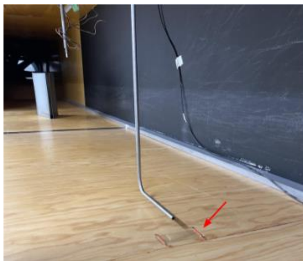
Figure 2.7. Co-located glycerol trap (indicated by red arrow) and dust intake tube.
