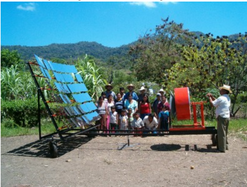
Figure 3.01. Fuego Solar Roaster. Roasting cacao in the Lacandon Jungle using pure sunlight with Don Flor turning the cacao and coffee roaster.
