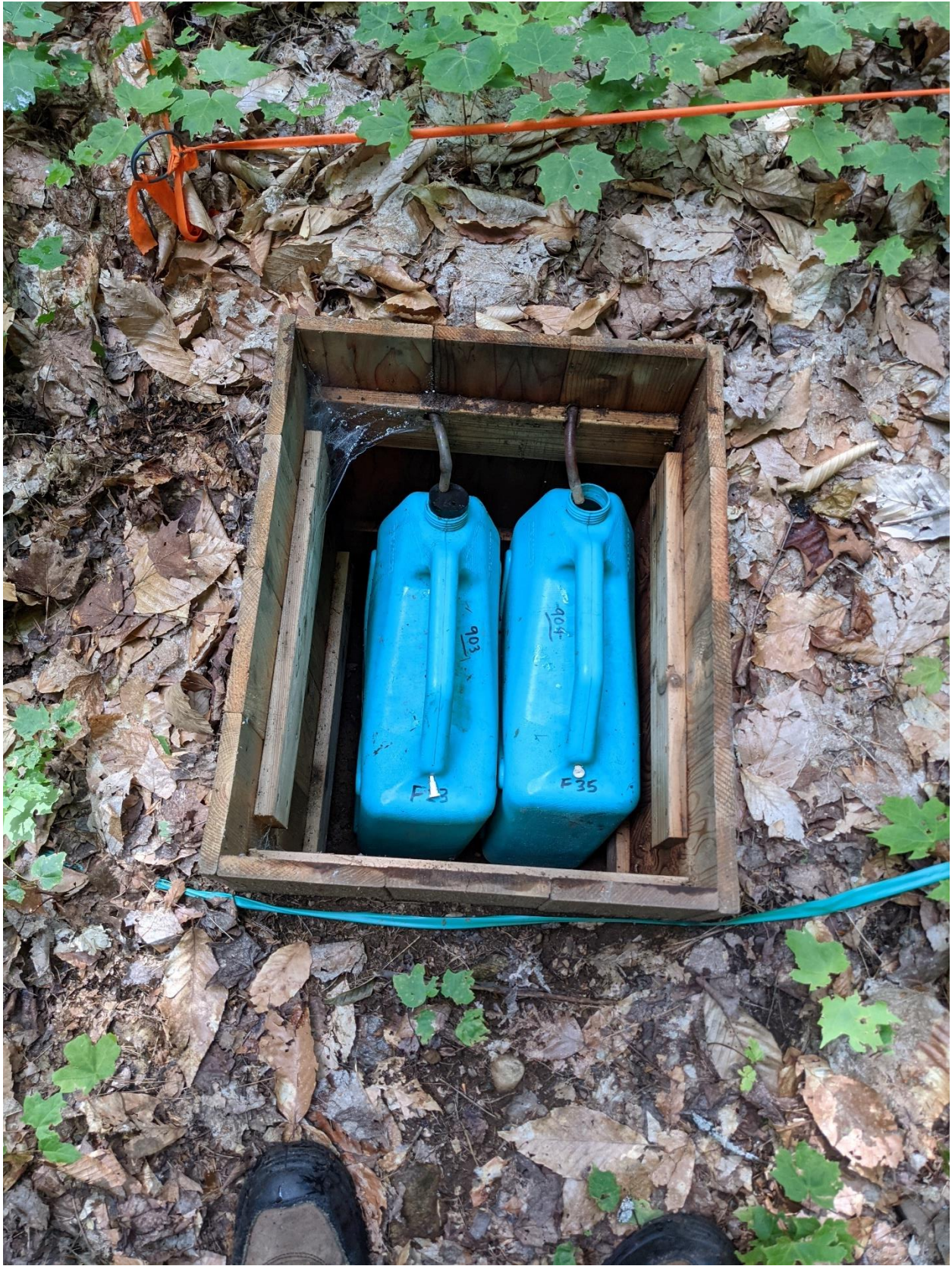
Figure 2.3 | Containment box for drainage and capturing soil water percolate from the LFH horizon at Porridge Lake, Ontario.
