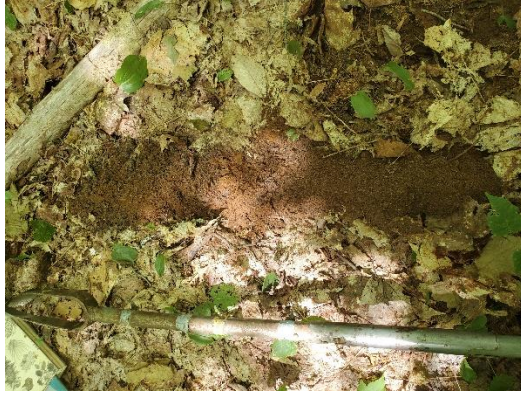
Figure 3.2 Site photograph of mineral horizon soil obtained using a Dutch auger, at Brookland farms.
