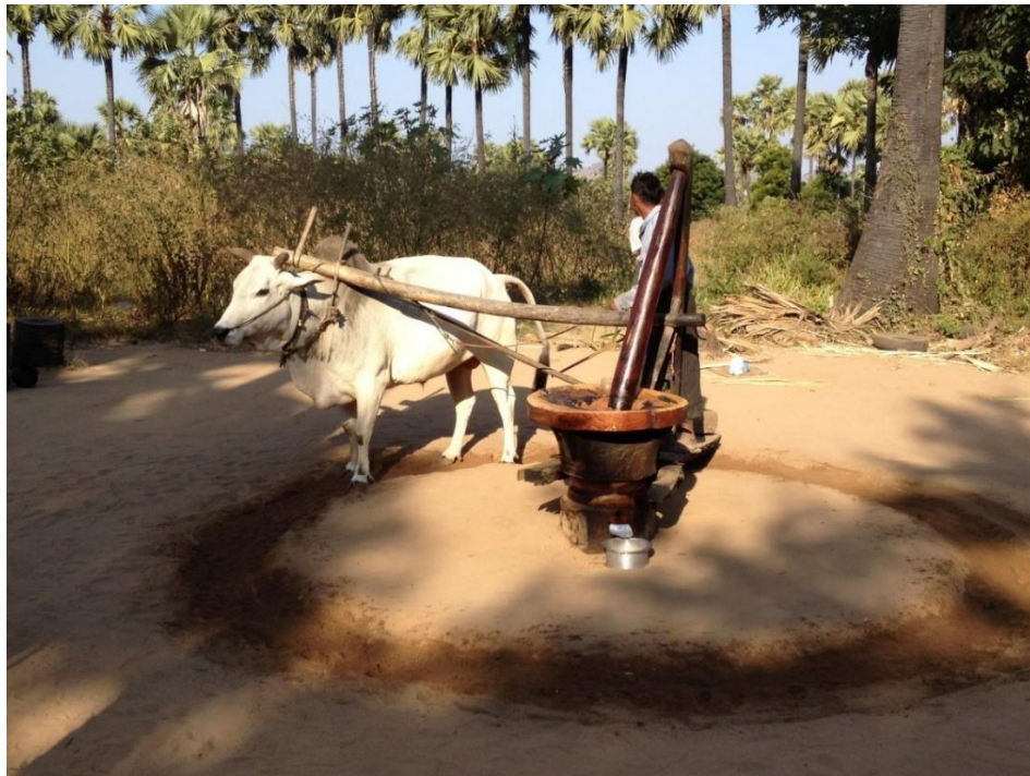
Figure 4.72. Cow powered peanut grinder at a toddy stop (Courtesy of Scott Macrae and the IRAW@Bagan Project).
